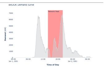
Resultant load profile due to modeled bus schedule, bus and charger type.
