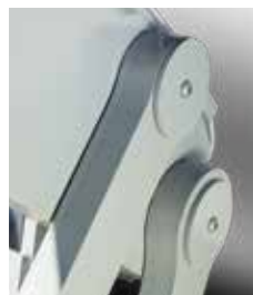
2" and 3" pins provide increased surface area to reduce loading on the pivoting members.
