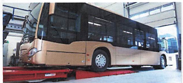
Fixed end-stops or "drive-thru" versions
