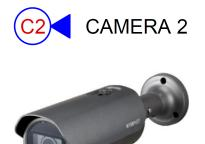
**XNF-9010RV**- Exterior Fisheye 12MP, Max resolution 3008x3008 @ 30FPS, 1.08mm fixed focal lends, Stereo graphic type lens, enhanced resolution for the peripheral regions, Fisheye, Single panorama, Double panorama, Quad view, on board dewarping, Digital PTZ, extreme WDR, Wise IR, IR, Video Analytics, Heatmap, People counting, Queue management, Hard coated dome cover, PoE, 12VDC
