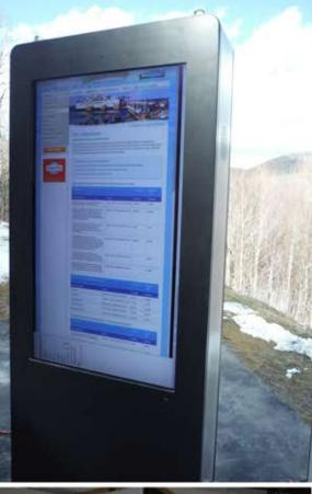
Single or Double Faced LCD units are specifically designed for outdoor use - ultra high brightness - 2000-2500 nit to compete with the direct sun.
